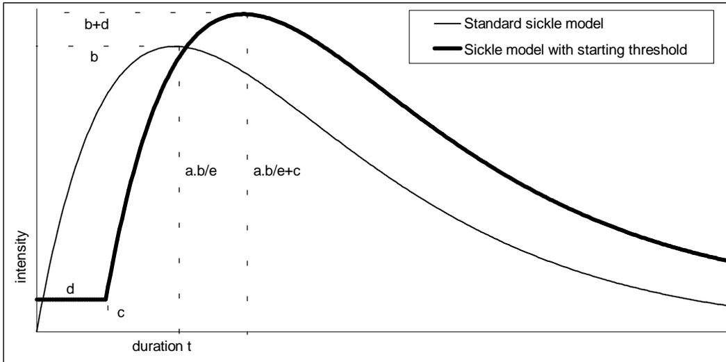
Figure 7: Standard sickle model, sickle model with starting threshold, and the meaning of their parameters
